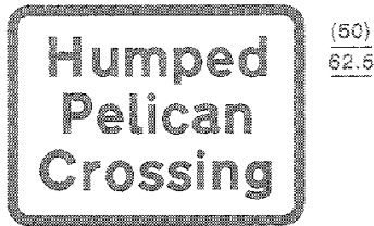
547.6 Pelican pedestrian crossing on road hump ahead
