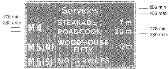
2917 Availability of motorway service areas ahead with distances and names of operators
