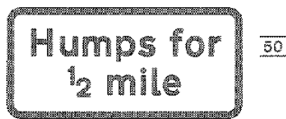
557.2 Road humps ahead for the distance indicated
