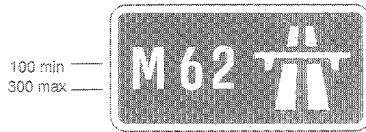
2901 Regulations in force under section 17 of the 1984 Act start to apply to the road at this point
