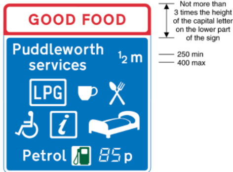
2919.1 Distance ahead to a named motorway service area at which fuel, parking, toilets and facilities for disabled persons are available, and refreshments, overnight accommodation, LPG fuel and a Tourist Information Point or Centre may be available, 24 hours a day throughout the year, and showing the name of the operator and the price per litre of unleaded petrol
