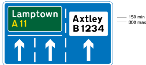
2913.3 The two left hand lanes of a motorway exit slip road lead to a primary route and the right hand lane leads to a non-primary route at a junction ahead
