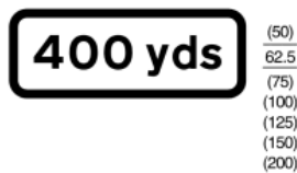
572 Distance ahead to hazard
