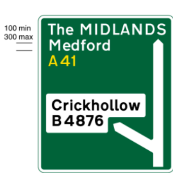
2014 Grade separated junction of a primary route with a non-primary route
