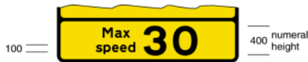
7275 Panel to appear at bottom of road works sign indicating temporary maximum speed in miles per hour advised
