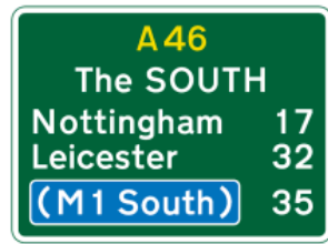
2030 The number of a primary route with distances to destinations along or reached from that route
