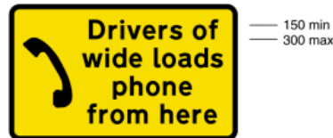
7293 Instructions to drivers of wide loads on location from which they should telephone for assistance
