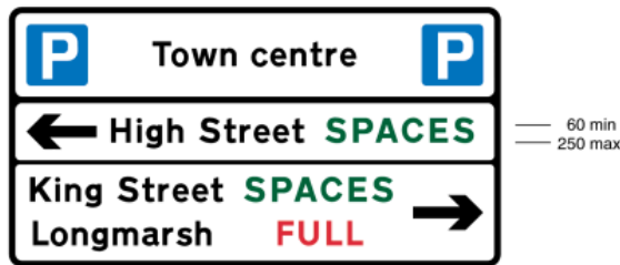
2509.1 Directions to several alternative parking places with an indication of the availability of parking spaces at each one (Variable message sign)
