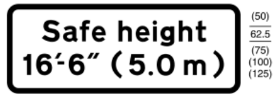
780A Safe height beneath electrified overhead cable ahead
