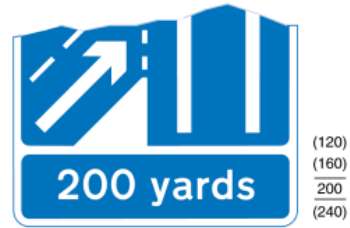
876 Distance to the change in the number of lanes indicated by the signs shown in diagrams 868 to 875
