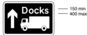
2929 Motorway junction ahead leading to a route advised for goods vehicles to the destination shown, which may differ from that for other traffic
