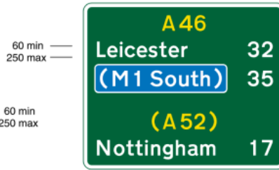
2030.1 Same as diagram 2030 but with the number of another primary route reached from that route and leading to a named destination
