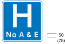
827.1 Hospital ahead without accident and emergency facilities
