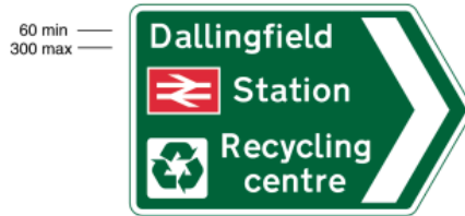
2027.1 Direction to a primary route which leads to the destination shown, to a railway station and to a recycling centre
