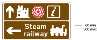
2216 Junction ahead leading to tourist attractions and a Tourist Information Point or Centre reached in different directions
