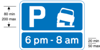
667.1 Vehicles may be parked partially on the verge or footway during the period indicated
