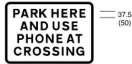
786 Place where large or slow, or long low vehicles should wait near a railway or tramway level crossing while the driver obtains permission by telephone to cross or confirms he has crossed
