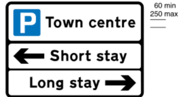
2505.1 Same as diagram 2505 with an indication of the general location of parking places
