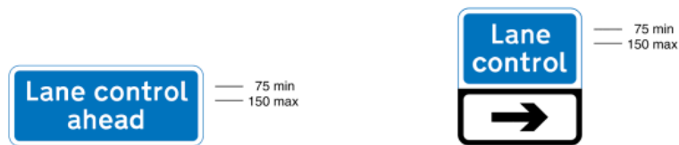
5012 System of lane control light signals ahead
