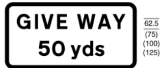
503 Distance to a junction ahead controlled by a diagram 602 ("GIVE WAY") sign
