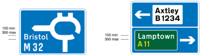
2913.1 Roundabout ahead leading from a motorway exit slip road to another motorway
