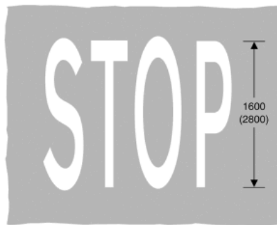
1022 Approach to a road junction or level crossing at or near which is placed the sign shown in diagram 601.1 and the road marking shown in diagram 1002.1
