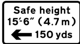
780.1A Safe height beneath electrified overhead cable in direction and at distance indicated
