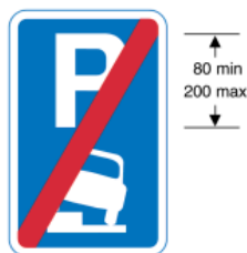
667.2 End of area where vehicles may be parked partially on the verge or footway
