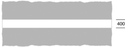
1002.1 Vehicular traffic must not proceed beyond the line when required to stop by the sign shown in diagram 601.1
