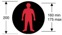
4006 Light signal at level crossing for pedestrians
