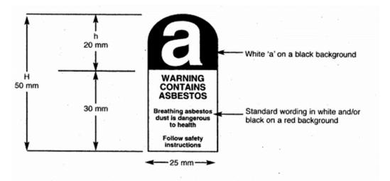
(2) In the case of a product containing crocidolite, the words "contains asbestos" shown in the diagram must be replaced by the words "contains crocidolite/blue asbestos".
