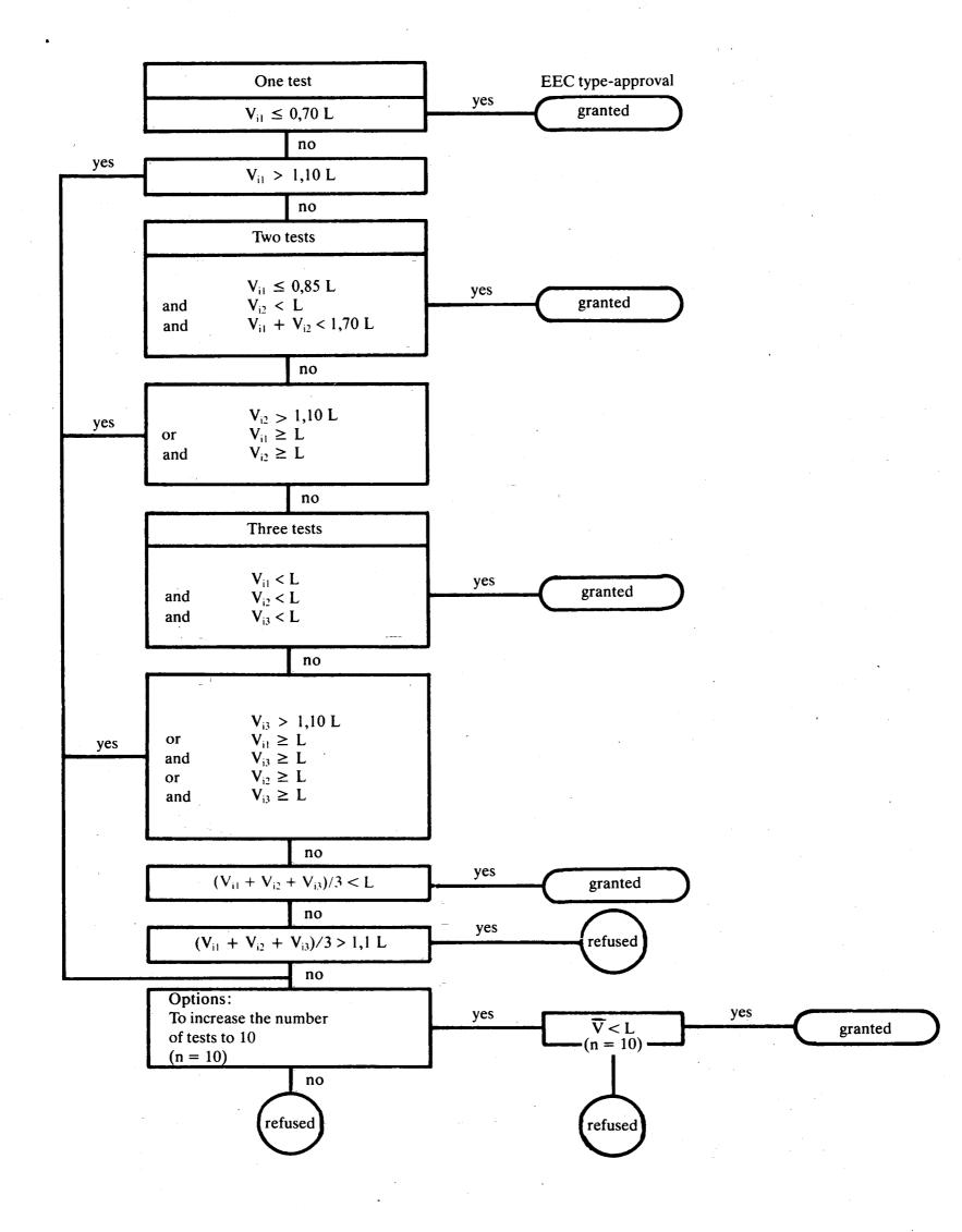
5.2.1.2. *Type II test* (carbon monoxide emission test at idling speed)
