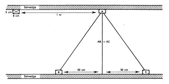
The thickness of the lines forming the sides of the rectangle must be 5 mm, and that of the diagonals 7 mm. The rectangle from the outer edge of the lines must be at least 8 cm in length and 5 cm in width.
