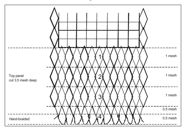
The distance of the window panel from the codline is 4 meshes. There are 3,5 diamond meshes in the upper panel and one 0,5 mesh deep hand-braided 'codline' row.
