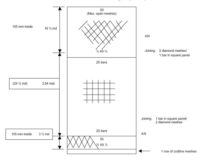
The construction of upper panel, size and position of the window panel in case when the escape panel runs from selvedge to selvedge
