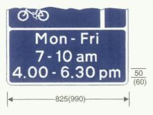
961 Times of operation of a bus lane or a cycle lane
