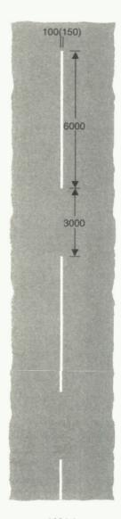
1004.1 As diagram 1004 on roads with a speed limit of more than 40 mph
