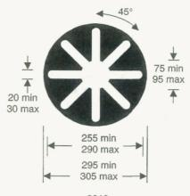
3013 Light signal for the control of tramcars
