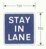
830.3 Vehicles should stay in lane for the purposes of a traffic survey or weight check ahead
