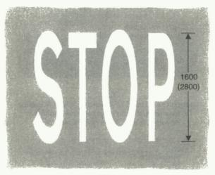
Approach to a road junction at or near which is placed the sign shown in diagram 601.1 and the road marking shown in diagram 1002.1
