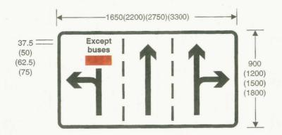
Junction ahead where the left hand lane is dedicated to traffic turning left and shall not be used by other traffic except buses and where the right hand lane is available both for traffic proceeding ahead and turning right
