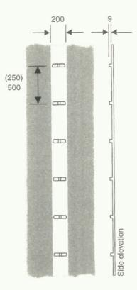
Alternative to the marking shown in diagram 1012.1 incorporating an audible and tactile warning in the form of a raised rib for use on motorways
