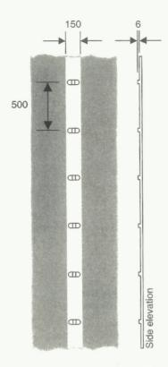
1012.3 As diagram 1012.2 for use on all-purpose roads with hard strips
