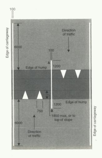
To indicate to vehicular traffic the presence of a flat top road hump extending across the whole width of a carriageway
