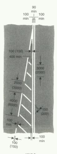
As diagram 1013.1, with an adjacent part of the carriageway which vehicular traffic should not enter unless it is seen by the driver to be safe to do so
