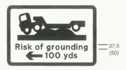
782.1 Risk of grounding at a railway or tramway level crossing or hump backed bridge
