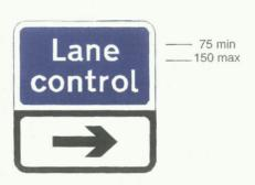
5013 Direction of a system of lane control light signals
