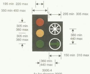
As for diagram 3000 with two additional signals as shown in diagram 3001, 3001.1 or 3013
