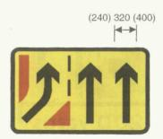
7254 Additional traffic lane joining from the left at a junction as part of temporary traffic management scheme
