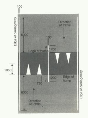
To indicate to vehicular traffic the presence of a round top road hump extending across the whole width of the carriageway
