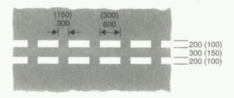
1003 Vehicular traffic shall give way in accordance with the requirements of regulation 24
