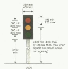
Light signals for the control of vehicular traffic at road junctions, at places where the headroom or width of the road is permanently reduced or at places where pedestrians, equestrians or cyclists cross the road (other than "Pelican" crossings)
