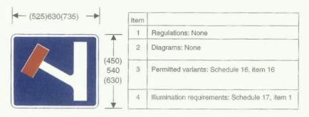
817 No through road for vehicular traffic in direction indicated from junction ahead
