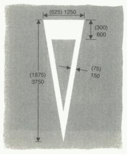
Approach to a road junction at or near which is placed the marking shown in diagram 1003 or both the marking shown in diagram 1003 and the sign shown in diagram 602
