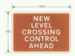
790 New method of controlling traffic at a railway or tramway level crossing ahead
