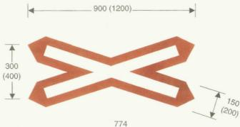
Location of railway or tramway level crossing without gate or barrier
