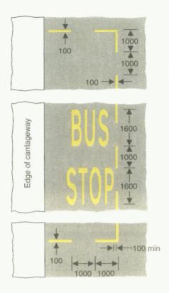
1025 Stopping place for buses on part of the carriageway also used by through traffic
