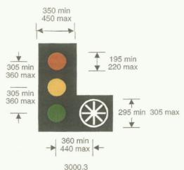
As for diagram 3000 with an additional signal as shown in diagram 3001, 3001.1, or 3013
