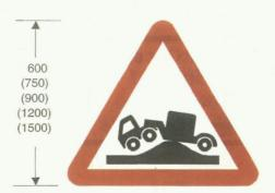
782 Risk of grounding at a railway or tramway level crossing or hump backed bridge
