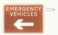
2708 Junction ahead leading to route for emergency vehicles to a temporary incident control point
