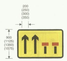
7202 Right hand two lanes of a four lane dual carriageway closed to traffic ahead
