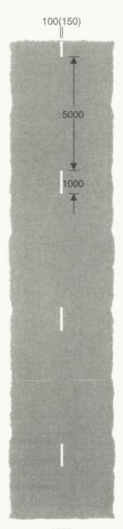
Division of the carriageway into traffic lanes on the part of the carriageway where vehicles normally proceed in the same direction on roads with a speed limit of 40 mph or less other than at places where the marking shown in diagram 1004 is used
