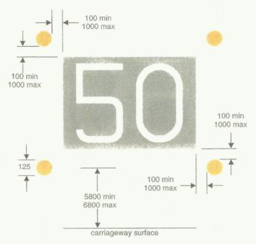
Gantry mounted signal with flashing amber lamps for displaying the signs shown in diagrams 6001, 6002, 6003, 6011 or 6011.1
