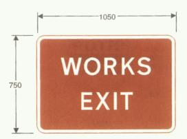
7302 Temporary exit from a construction or roadworks site
