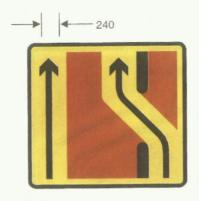
7216 Right hand lane returns to right hand side of original carriageway ahead, but remains separated by works area from left hand lane
