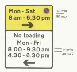
Waiting prohibited during the period and in the direction indicated on the upper portion and loading and unloading prohibited during the period and in the direction indicated on the lower portion
