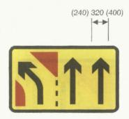
7250 Near side traffic lane diverges from main carriageway at a junction as part of temporary traffic management scheme
