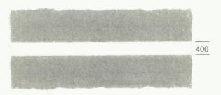
1002.1 Vehicular traffic shall not proceed beyond the line when required to stop by the sign shown in diagram 601.1
