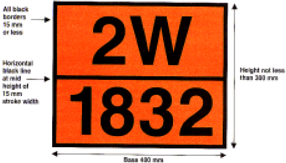
Orange-coloured panel displaying the emergency action code and the UN number
