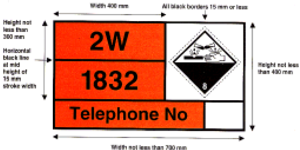
Hazard warning panel
