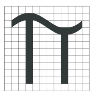
If the marking is reduced or enlarged, the proportions of the drawing must be respected.
