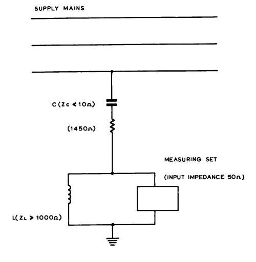
CIRCUIT FOR RE VOLTAGE MEASUREMENT
