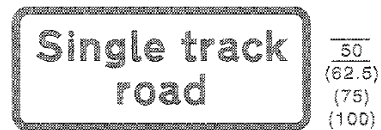
519 Road only wide enough for one line of vehicles
