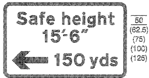
780.1 Safe height beneath electrified overhead cable in direction and at distance indicated
