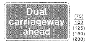
818 Section of dual carriageway road begins directly ahead
