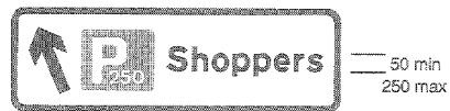
2506 Direction to a parking place for shoppers and showing the total number of parking places
