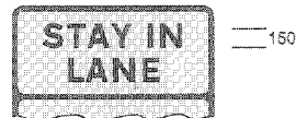
7263 Panel to appear at top of road works sign instructing traffic to remain in appropriate lane
