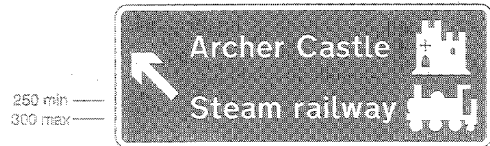
2924 Motorway junction ahead leading to the tourist attractions shown
