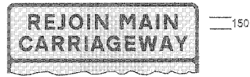
7261 Panel to appear at top of road works sign instructing traffic using hard shoulder to rejoin main carriageway
