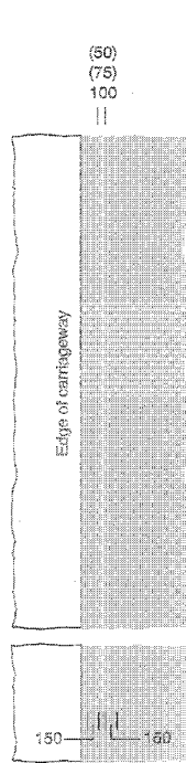
1017 Waiting of vehicles on a side of a length of road prohibited for a time less than that specified in the caption to diagram 1018.1
