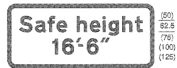
780 Safe height beneath electrified overhead cable ahead
