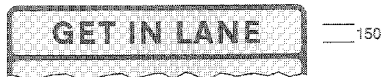
7262 Panel to appear at top of road works sign instructing traffic to get into the appropriate lane as indicated on main part of sign
