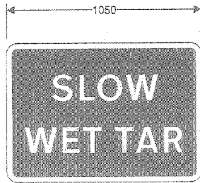
7010 Vehicular traffic should proceed slowly owing to temporary hazard resulting from wet tar on the road
