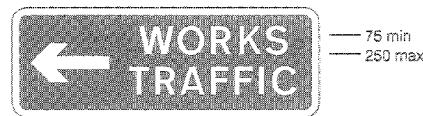
7304 Direction to be taken by road works or construction traffic at a junction or works entrance ahead
