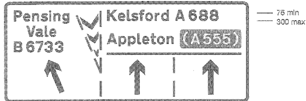
2115.1 Grade separated junction where one lane of a non-primary route is reserved for traffic turning onto another non-primary route
