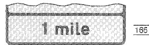
7270 Panel to appear at bottom of road works sign indicating distance in miles to junction indicated on signs shown in diagrams in item 3 of the table
