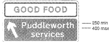
2920 Direction to a named motorway service area and showing the name of the operator
