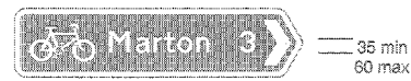
2602 Direction and distance to destination shown of route recommended for pedal cycles, which differs from that for other traffic
