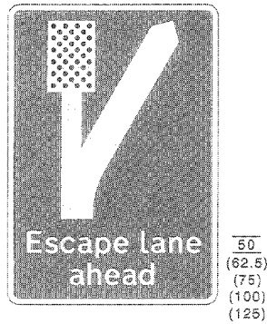
817.2 Escape lane ahead for vehicles unable to stop on steep hill
