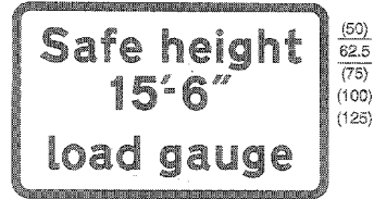
780.2 Safe height beneath electrified overhead cable ahead provided with a load gauge shown in diagram 781
