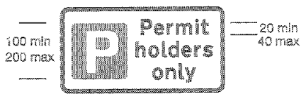
660 Parking place reserved for permit holders
