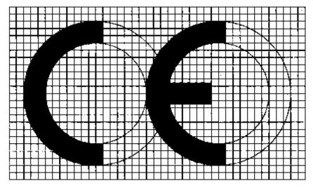
If the CE marking is reduced or enlarged the proportions given in the above graduated drawing must be respected. The different elements of the CE marking should have materially the same vertical dimensions which should not be less than 5mm."
