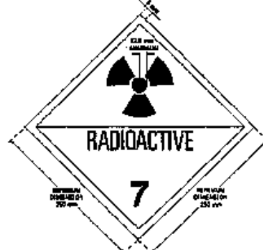
Fig. 5. Placard. Minimum dimensions are given: when larger dimensions are used the relative proportions must be maintained. The figure "7" shall not be less than 25 mm high. The background colour of the upper half of the placard shall be yellow and the lower half white, the colour of the trefoil and the printing shall be black. The use of the word "RADIOACTIVE" in the bottom half is optional to allow the alternative use of this placard to display the appropriate United Nations Number for the consignment.
