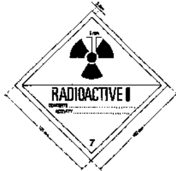
Fig. 2. Category I-WHITE label. The background colour of the label shall be white, the colour of the trefoil and the printing shall be black, and the colour of the category bar shall be red.
