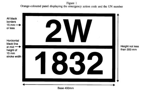
Figure 2 Hazard warning panelThe emergency action code shall be inscribed in the upper half and the UN number in the lower half of the orange-coloured panel and the telephone number beneath the UN number.
