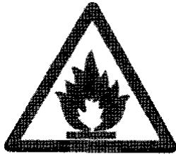
Flammable material or high temperature (a)
