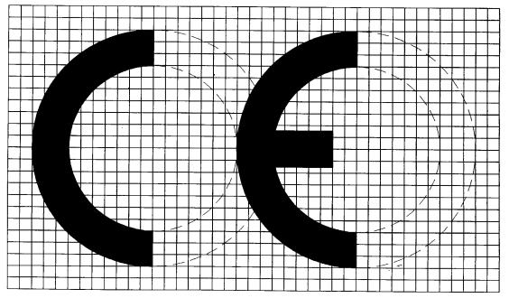
If the CE marking is reduced or enlarged according to the size of the equipment the proportions given in the above drawing must be respected. The various components of the CE marking must have substantially the same vertical dimensions which may not be less than 5 mm.
