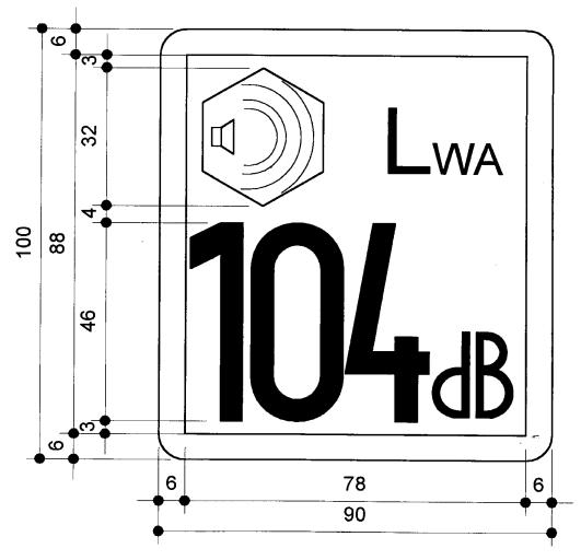
If the indication is reduced or enlarged according to the size of the equipment the proportions given in the above drawings must be respected. However, the vertical dimension of the indication should, if possible, not be less than 40mm.
