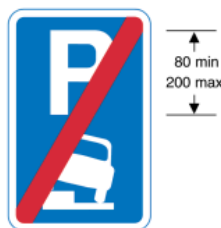
667.2 End of area where vehicles may be parked partially on the verge or footway
