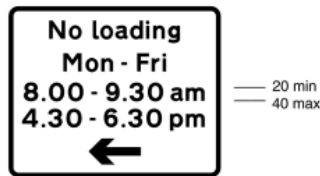
638.1 Loading and unloading prohibited during the periods and in the direction indicated
