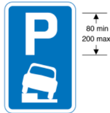
667 Vehicles may be parked partially on the verge or footway
