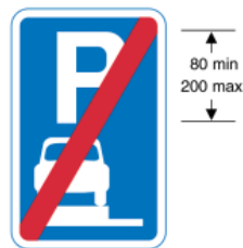
668.2 End of area where vehicles may be parked wholly on the verge or footway
