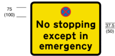
642.3 No stopping in lay-by except in emergency
