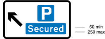
2511 Direction to a secured car park approved by the police under the ACPO secured car park scheme
