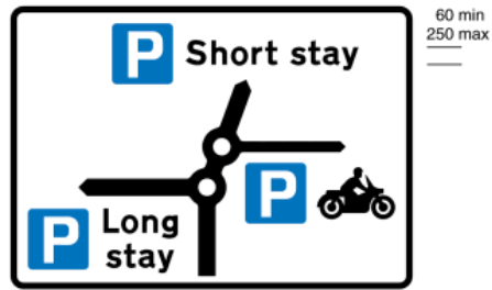
2513 Double mini-roundabout ahead with exits to three different types of parking place
