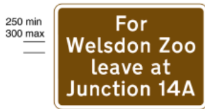
2927.1 Exit from a motorway at a junction ahead that should be used for a tourist attraction that is not otherwise shown on signs on the main carriageway of the motorway at that junction
