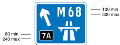
2902.1 Direction to a motorway at the junction shown, indicating route number
