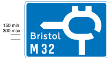
2913.1 Roundabout ahead leading from a motorway exit slip road to another motorway
