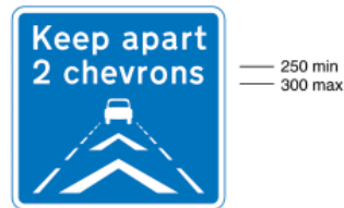
2933 Drivers should keep a distance of two chevron markings from the vehicle in front
