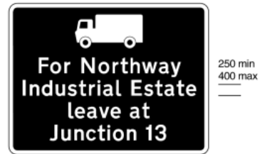
2929.1 Exit from a motorway at a junction ahead that should be used for a destination along a route advised for goods vehicles that is not otherwise shown on signs on the main carriageway of the motorway at that junction
