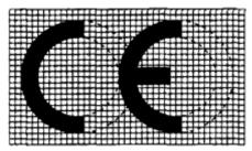
If the CE marking is reduced or enlarged the proportions shown in the above drawing must be respected.
