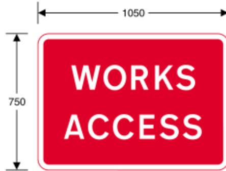
7301 Temporary access to a construction or road works site
