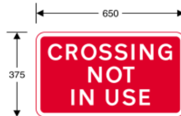
7016 Zebra or signal-controlled crossing facility temporarily out of use (Sign for pedestrians, cyclists or equestrians)
