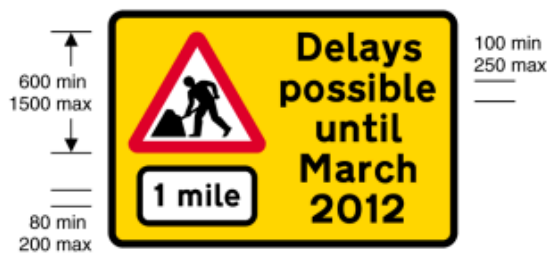
7005 Delays possible for specified period owing to road works ahead
