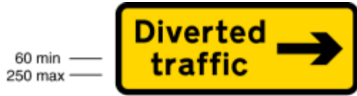
2703 Direction of temporary diversion route from junction ahead
