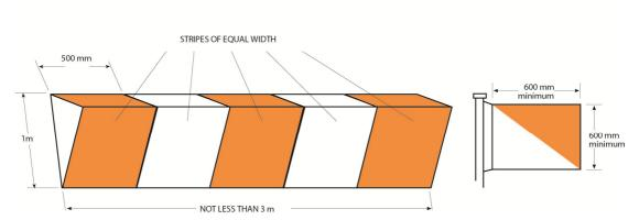
indicate the boundary of an area unfit for the movement of aircraft.
